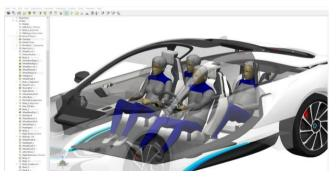
Figure 1: RAMSIS Software can be used e.g. for occupant packaging studies
